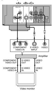
If your AV amplifier has video output terminals, connect your amplifier (and then to your video monitor) so that you can use one video monitor for several different video sources (LD, VCR etc.) by simply switching the input source selector of your amplifier.
