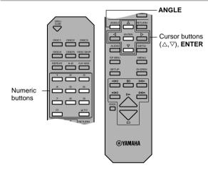
Some DVDs have scenes encoded with multiple camera angles so that different viewpoint can be selected during playback. ANGLE lights up on the front panel display while a scene encoded with multiple angles is being played.
