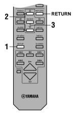
This section shows common procedures (some items require additional steps). Use the remote control to operate the setup menu.
