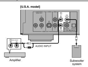
Connect AUDIO OUT L (left) and R (right) terminals of this unit to corresponding input terminals of your audio equipment such as stereo amplifier.
