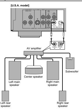
This unit has COAXIAL and OPTICAL digital output terminals. Connect one or both of them to your AV amplifier equipped with Dolby digital, DTS, or MPEG decoder using each specific cable (separate purchase).
